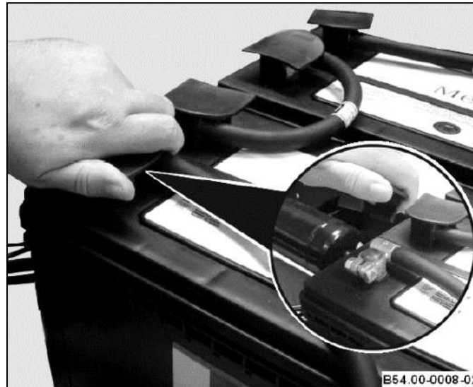
Battery connector protection cover B54.00-0008-02
